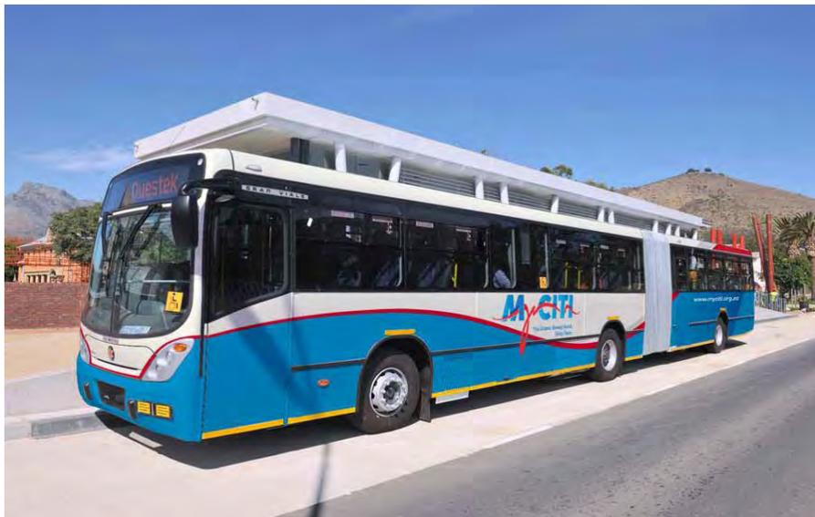
**Figure 11: 18m Articulated trunk vehicle**
