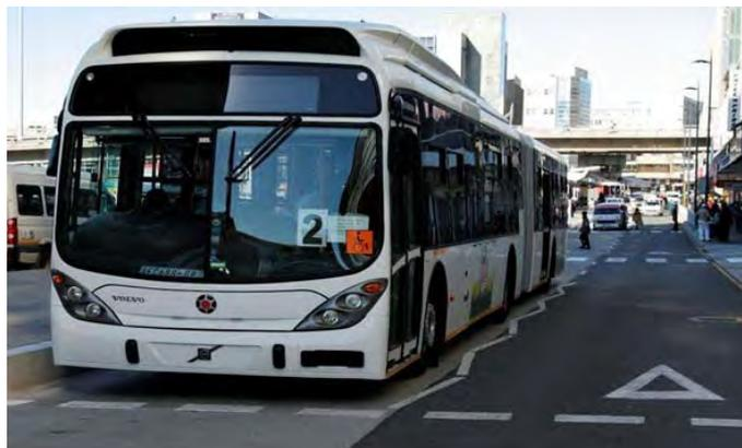
**Figure 12: Example of a 18m articulated low-floor vehicle**
