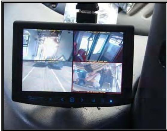
**Figure 32. The Driver's CCTV display**
