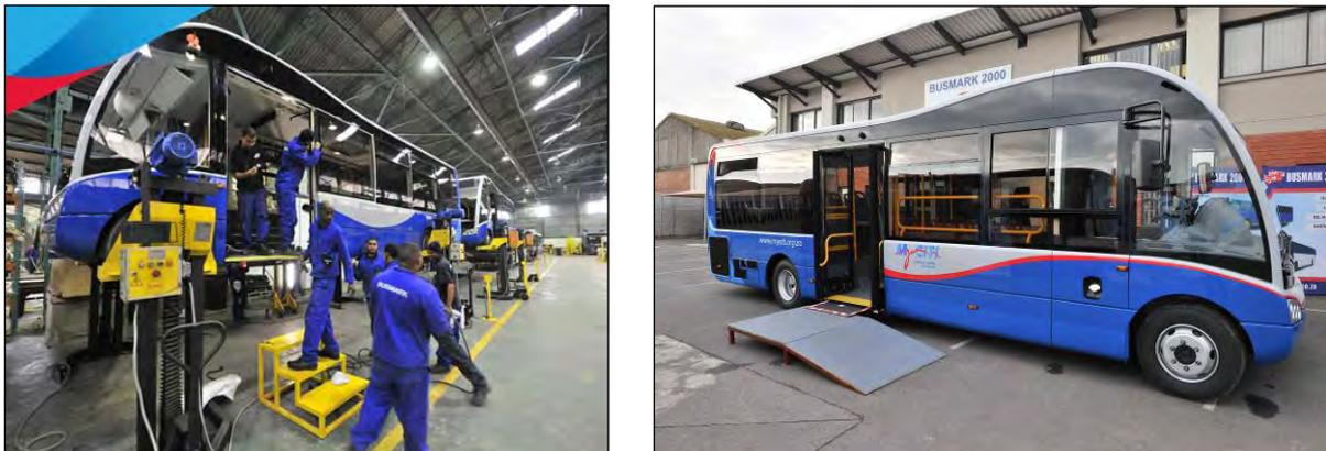
**Figure 25. Optare SR buses on the assembly line in Elsie's River and a completed feeder service bus finished in the MyCiTi livery**
