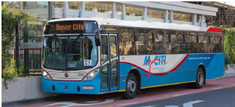
**Figure 10: 12m Solo trunk vehicle**
